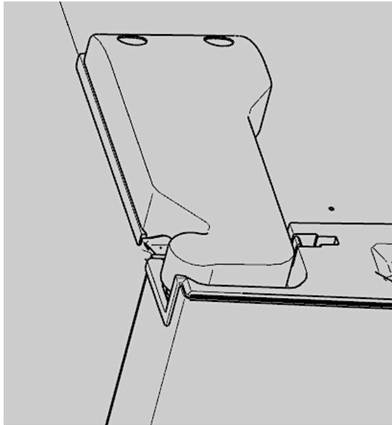
21. Install the door magnet (s. step 7.) on the left side of the appliance door.
