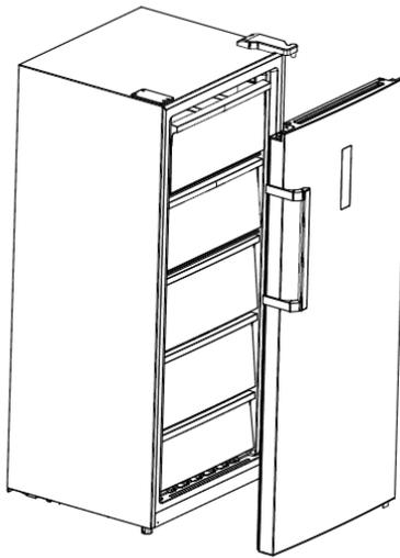
11. It is necessary to tilt the appliance backwards. Lean the appliance against a solid and immovable surface so it will not slip. **Do not** tilt the appliance more than **45°**.
