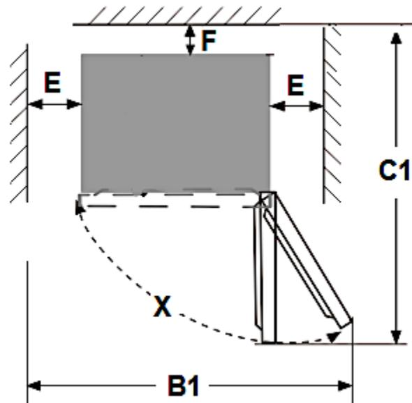
$$B1 = \text{WIDTH} + 2 \cdot E / C1 = \text{DEPTH} + F / X = \text{DOOR OPENING ANGLE}$$
