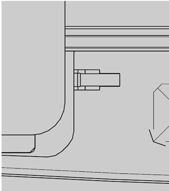
22. Install the door handle on the **right** side of the appliance door; refer to chapter 3.4 INSTALLATION OF THE DOOR HANDLE. To install the door handle on the right side of the appliance, you must turn it through 180°.
