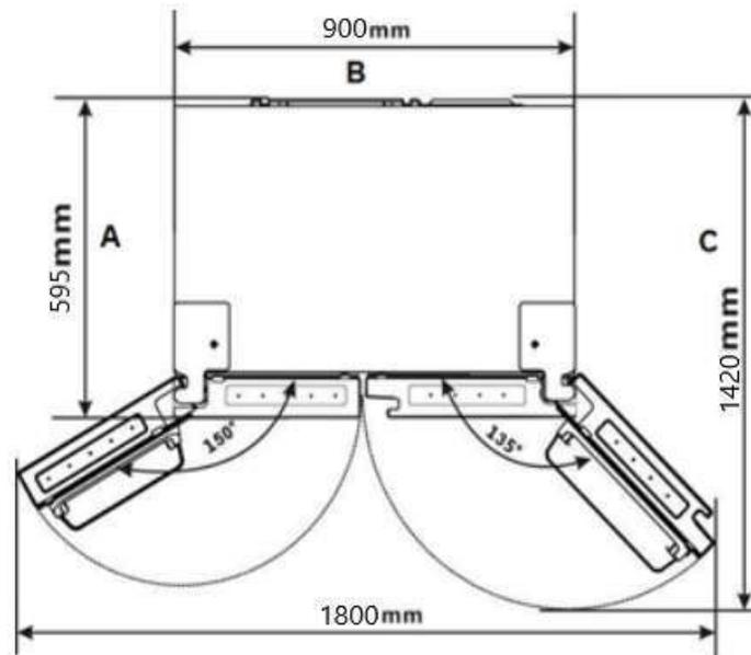
**A = DEPTH / B = WIDTH / C = DEPTH (WHEN THE DOOR IS OPEN)**
