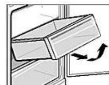
**i** The freezer drawers can be removed and installed for cleaning as shown above.
