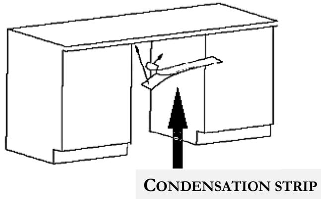
**NOTICE!** Improper installation of the condensation strip may cause damage to the worktop.
