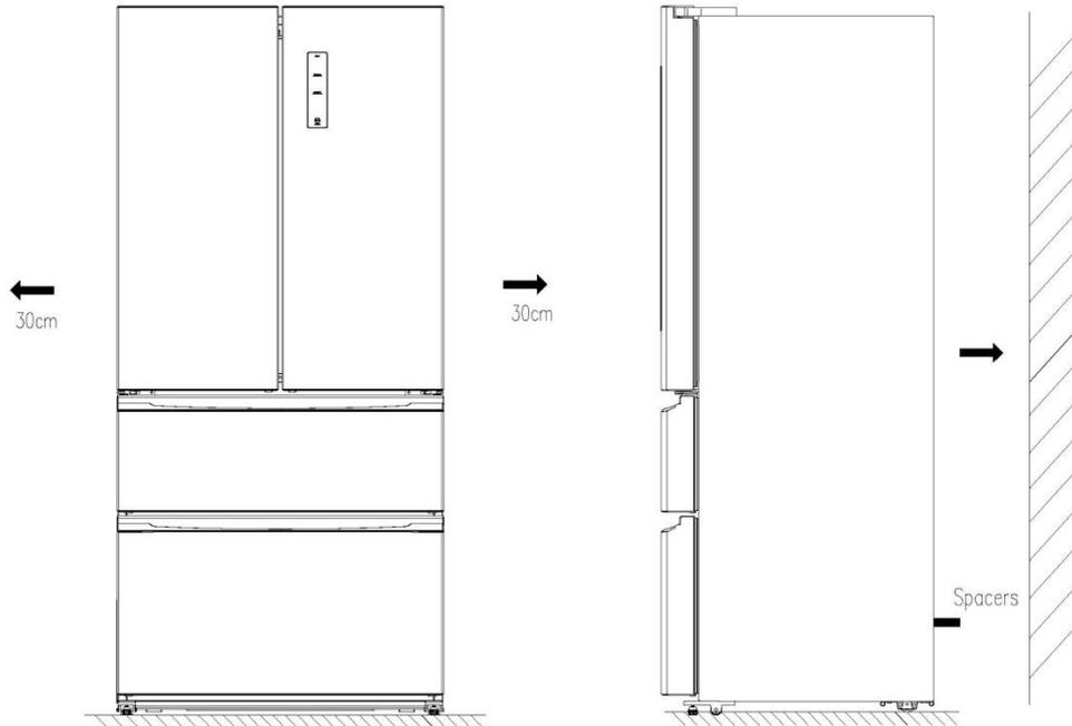
**i** Observe the required minimum distances for proper ventilation.
