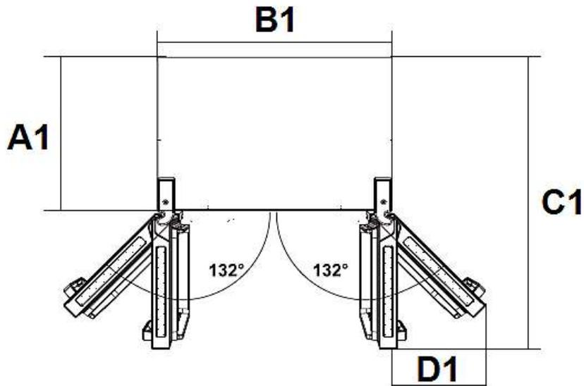
**A 1 = Depth / B 1 = Width / C 1 = Depth (when the doors are open) /
