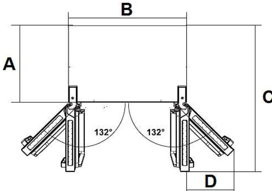
**A = Depth / B = Width / C = Depth ( when the doors are open) / D = Space requirement of the doors**
