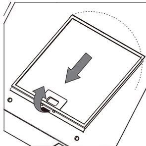
3. Plug the carbon filter into the appliance and turn in clockwise direction.
