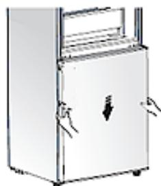
28. Align the middle door hinge (**J**) to the prepared holes on the left side of the appliance properly; s. fig. below (it may be necessary to turn the middle hinge
