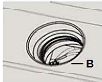
4. Install the water tank on the door. Ensure that the sealing ring has been inserted into the appropriate opening before. Hold both sides of the water tank tightly. Insert the water valve into the appropriate opening and install the water tank at an angle of 45°.
