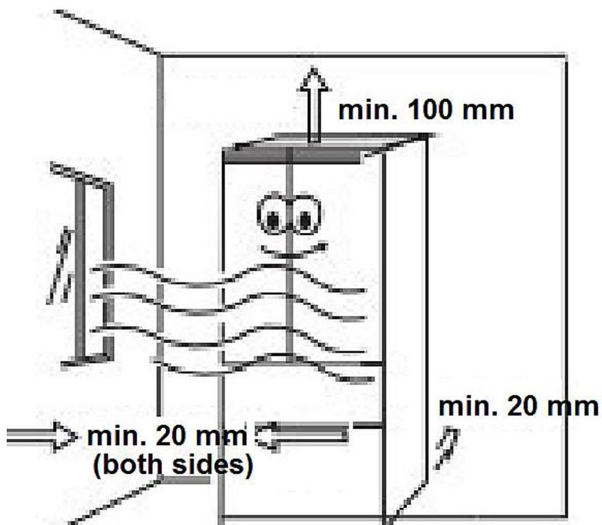
**SPACE REQUIREMENT OF THE APPLIANCE INCL. MINIMUM DISTANCES FOR PROPER VENTILATION**
