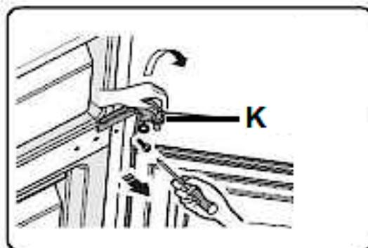
11. Lift the freezer door and remove it carefully (s. fig. below). Place the freezer door on a smooth surface with the external cladding facing up.
