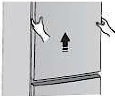
7. Unscrew the door holder (**F**) and the right door block (**G**) of the fridge door (s. fig. below). Store the **right** door block (**G**) in the accessory bag.
