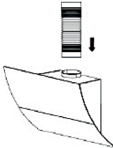
8. Insert the upper chimney (5) into the lower chimney (4). Fix the lower chimney bracket on the lower chimney at the desired height using two 4\*8 mm screws (s. fig. below). Do not tighten the screws too firmly so the upper chimney will stay telescopic after installation.
