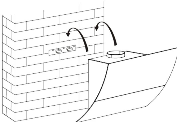
3. Four additional 4\*8 mm drillings are required to fix the appliance.
