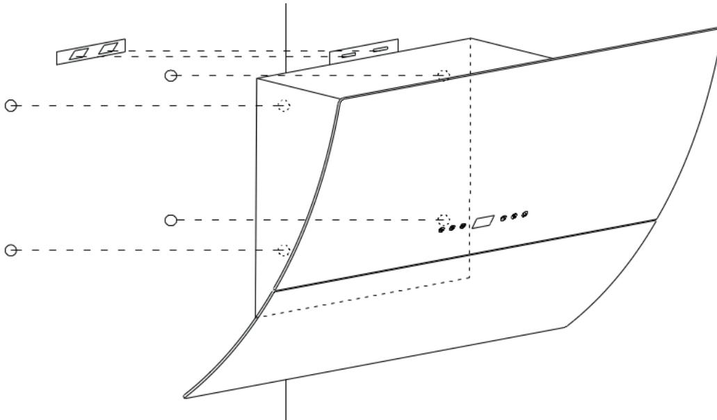
4. Lift the extractor hood (2) and hang it on the wall bracket (1) again (s. fig. below).
