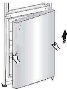
16. Remove the screw hole cover (K) of the middle door hinge from the left side of the appliance and install it on the opposite side (right); s. fig. below.
