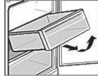
**i** Any of the freezer drawers can be removed and reinserted for cleaning as shown above.<sup>21</sup>
