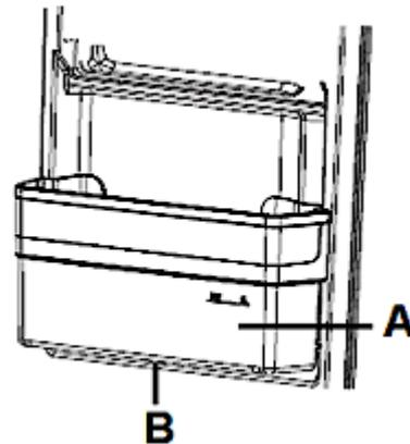
5. Place the water tank in proper position by pushing it downwards slightly and carefully until the water tank is seated properly in the door of the appliance.
