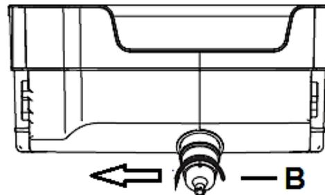
3. First, push the connector / flange of the cover (E) of the water tank on **one** side of the water tank upwards slightly and carefully to separate the **cover (E)** of the water tank from the water tank (A) itself. Then repeat the procedure on the other side of the water tank. Remove the cover from the water tank.
