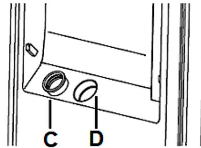
c) Insert the sealing ring (C) into the opening (D) properly again.
