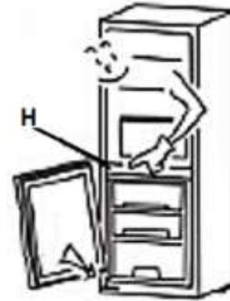
7. Place the fridge-door on the middle hinge; the hinge pin must be inserted in the hole on the bottom of the fridge-door. Close the door, then install the top hinge on the opposite side. The top hinge pin must be inserted in the hole on the top of the fridge-door. Install the hinge cover.
