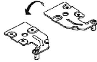
12. Remove the left screw hole cover (1) and install the right screw hole cover (2/in the plastic bag).
