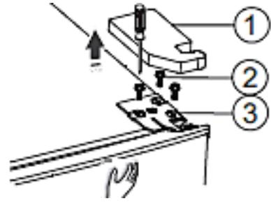
3. Remove the upper door. Place the door on a soft base with the panel up. Unscrew the screws (1) and remove part 2. Then install part 2 on the opposite side using the screws (1).
