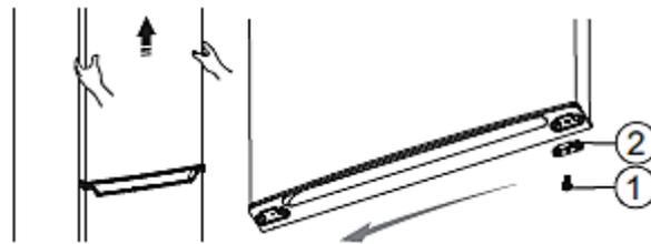
4. Unscrew the screws (1) of the middle hinge (2) and remove the middle hinge; then remove the lower door.
