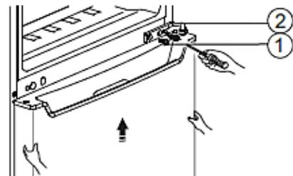
5. Place the door on a soft base with the panel up. Unscrew the screws (1) and remove part 2. Then install part 2 on the opposite side using the screws (1).
