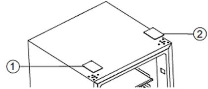
13. Move the door to installation position. Align part 1 and the door. Then fix part 1 using the screws (2). Hold the top door during work. Install part 3 (in the plastic bag). First push part 3 from the left to the right completely; then press downwards.
