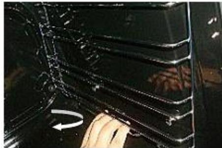
3. To remove the side rack, hold it to the oven horizontally.
