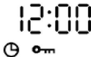
11. As soon as the temperature in the oven is **less than 300 °C**, the **door locking** of the appliance will be **deactivated**. The indicator of the door locking «
