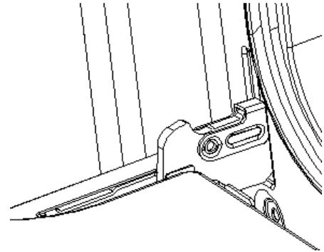
4. **If the safety catch is not closed properly you will damage the hinges when closing the door.**
