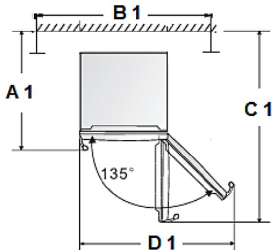
**A 1 = Depth / B 1 = Width / C 1 = Depth (when the doors are open) /
