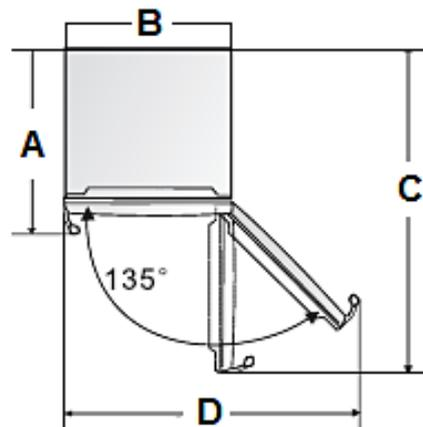
**A = Depth / B = Width / C = Depth (when the doors are open) / D = Space requirement of the appliance (width) when the doors are open / door opening angle 135°**
