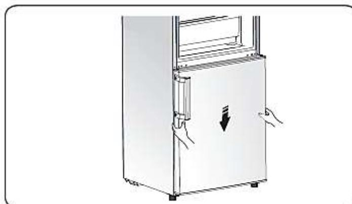
33. Turn the middle door hinge (H) through 180°. Align the middle door hinge (H) to the prepared holes on the left side properly (s. fig. below). While doing so, insert the hinge axis of the middle door hinge into the upper hinge hole of the freezer door. Screw the hinge using the self-tapping screws (I); s. fig. below.
