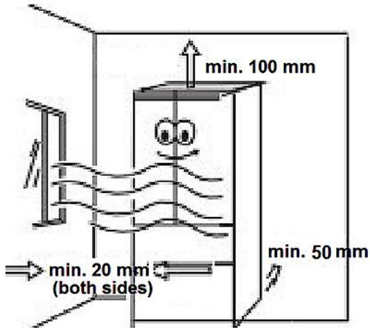
**SPACE REQUIREMENT OF THE APPLIANCE WHEN THE DOORS ARE CLOSED (INCL. MINIMUM DISTANCES FOR PROPER VENTILATION)**
