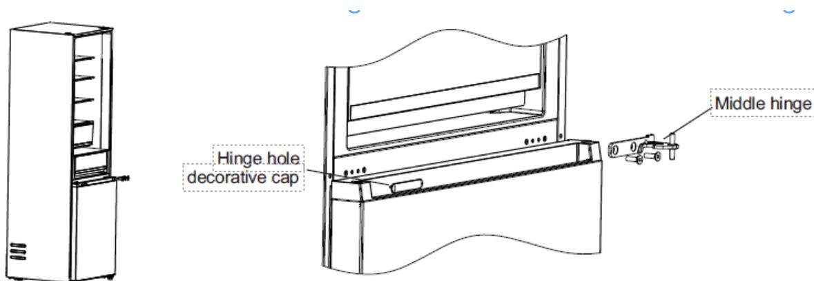
4) Remove the refrigeration door body (pay attention to the small parts such as shaft sleeve and stop on the door, make sure they are not to be lost); Remove the lower hinge and leveling foot. Remove the lower hinge stop and the hinge shaft and install them on the other side of the hinge, and install the modified lower hinge on the other side of the refrigerator; The leveling foot is installed on the original hinge side.
