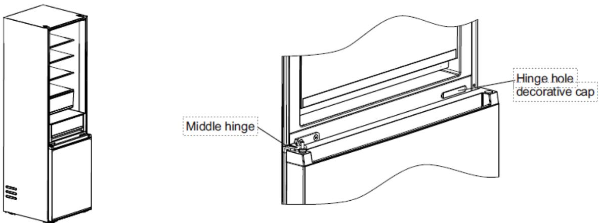
8) Place the refrigeration door body on the middle hinge and install the upper hinge; Connect the refrigerator top signal 4 with the door body signal line 1. Finally, the hinge cover is installed at the left hinge; The hinge cover decorative cap is installed at the top of the right side.
