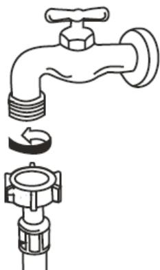
3. Put the other end of the water inlet hose into a bucket or into another suitable container (s. fig on the right) and open the water tap to flush foreign substances (e.g., dirt, sand, etc.) out of the water pipe and of the hose. Check the water temperature.
