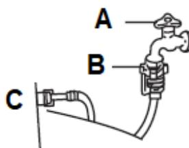
4. Remove the hose and immerse it in warm water (approx. 50 °C / s. fig. below).
