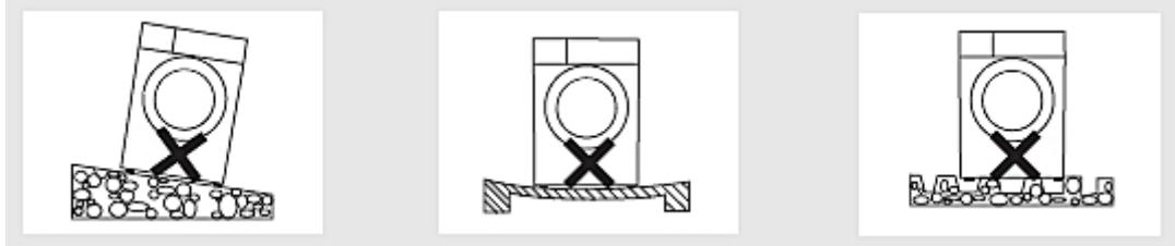
11. If you install the appliance on a wooden floor, you must also place it on a plywood panel (60.00\*60.00 cm) **at least** 3.00 cm thick to distribute the weight of the appliance. Fix and secure the plywood panel properly to the wooden floor.
