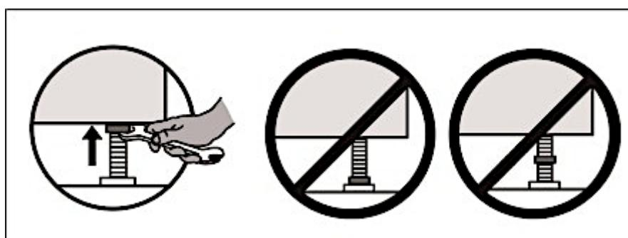
**NOTICE! Do not turn the adjustable feet out further than absolutely necessary!** The further the adjustable feet are turned out, the more the appliance may vibrate.
