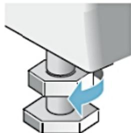
b. How to tighten the lock nut: turn the lock nut anti-clockwise (s. fig. on the right). Use the spanner provided.
