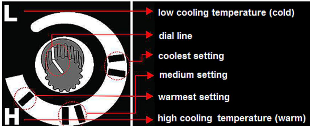
7. The setting unit is on the back of the appliance.
