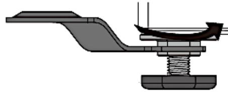
3. Turn the adjustable feet for horizontal alignment.
