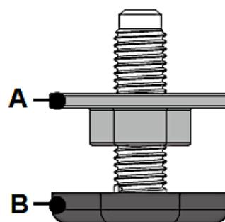
a. How to **loosen** the lock nut: turn it to the **left** using the spanner (s. fig. on the right).
