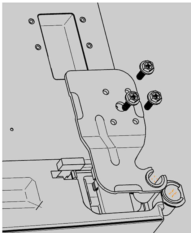
8. Insert the door communication wire into the opening on the door and install the cover.
