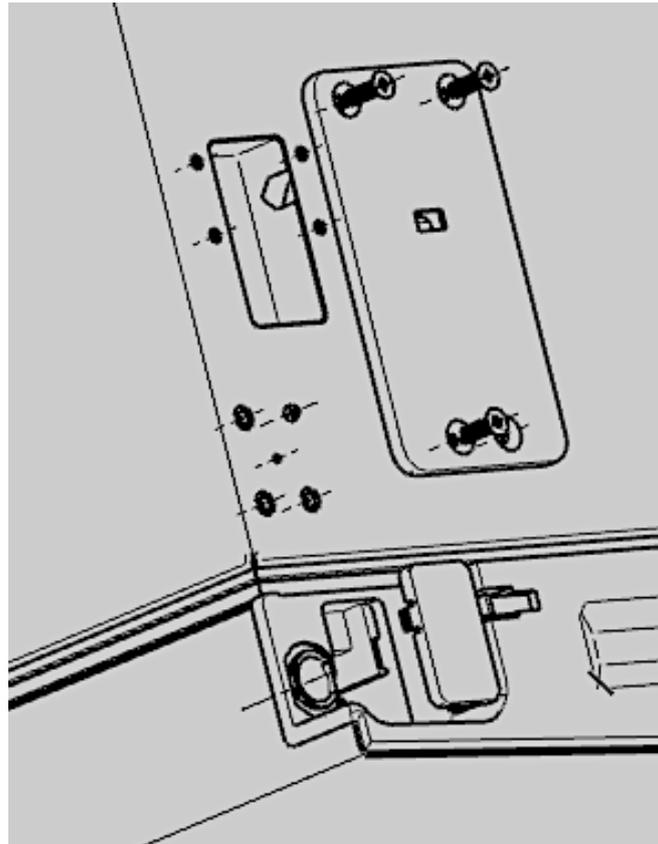
10. Lift the door of the appliance and remove it carefully. Place the door on a smooth surface with the external cladding facing up.
