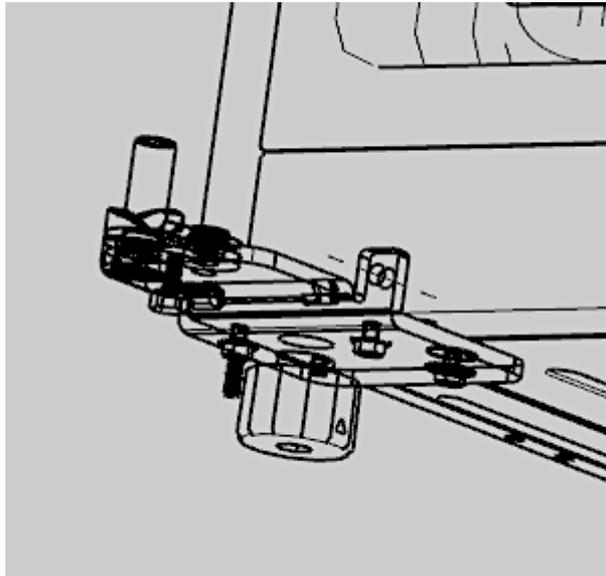
14. Unscrew the right door block on the bottom of the appliance door and keep it in a safe place. Take the **left door block** from the plastic bag and install it on the bottom left side of the appliance door accordingly.
