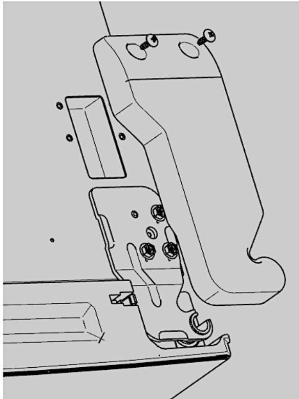
6. Unscrew the top right door hinge and remove it. Keep the top right door hinge cover and the top right door hinge in a safe place.
