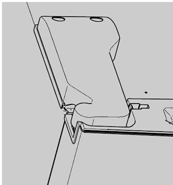
21. Install the door magnet (s. step 7.) on the left side of the appliance door.
