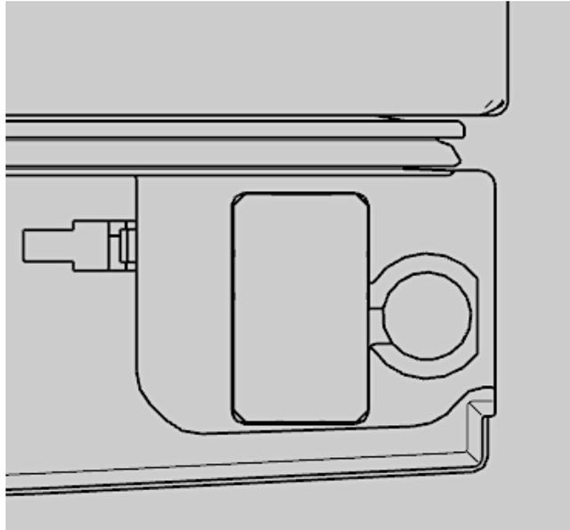
9. Remove the top screw hole cover on the left side of the appliance door. Unscrew the left cover and remove it. Remove the wire harness from the opening and install the door sleeve (s. step 7.).
