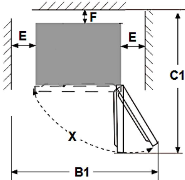
$$B1 = \text{WIDTH} + 2 \cdot E / C1 = \text{DEPTH} + F / X = \text{DOOR OPENING ANGLE}$$
