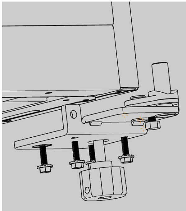
13. Take the **bottom left door hinge** from the plastic bag. Align the door hinge with the holes on the bottom left side of the appliance properly and screw it tight. Reinstall the adjustable feet.
