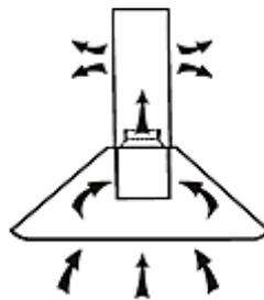
2. You can use carbon filters for odour absorption in recirculation mode only. For installing carbon filters, remove the grease filter. Press the lock and pull the grease filter downwards.
