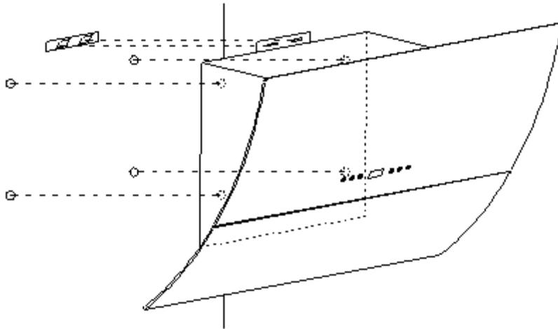
3. Hang the appliance on suspension bracket. Fix the appliance (look at step 2). The appliance must be installed in horizontal position. Check proper position using a spirit level.
