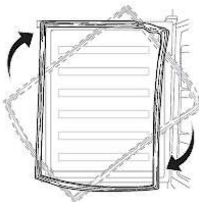
27. Install the freezer door on the bottom door hinge. For this purpose, insert the hinge pin of the bottom door hinge into the bottom hinge hole of the freezer door carefully. Hold the door in position (s. fig. below).
