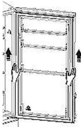
14. Unscrew the middle door hinge(J); s. fig. below. Meanwhile, hold the freezer door with your hand so it cannot drop down.
