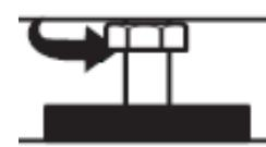
**NOTICE!** After you have levelled the appliance properly, always tighten the lock nuts again.
