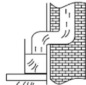
**Horizontally:** Lay the exhaust hose to an exhaust outlet equipped with an air grille\*.
