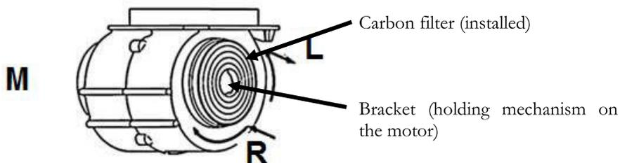
L Turn to the left = Remove a previously installed carbon filter.
