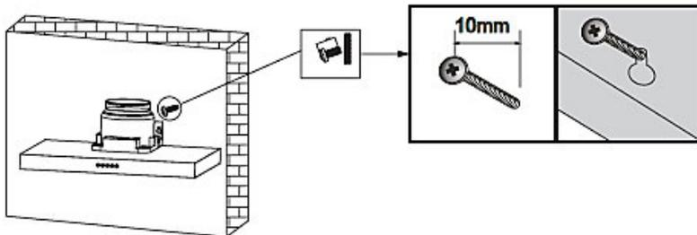
3. Tighten the four screws; start with the upper two screws, then tighten the lower ones.
