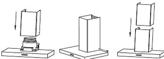
6. Adjust the two chimneys relevant to the dimensions of the fixing bracket.
