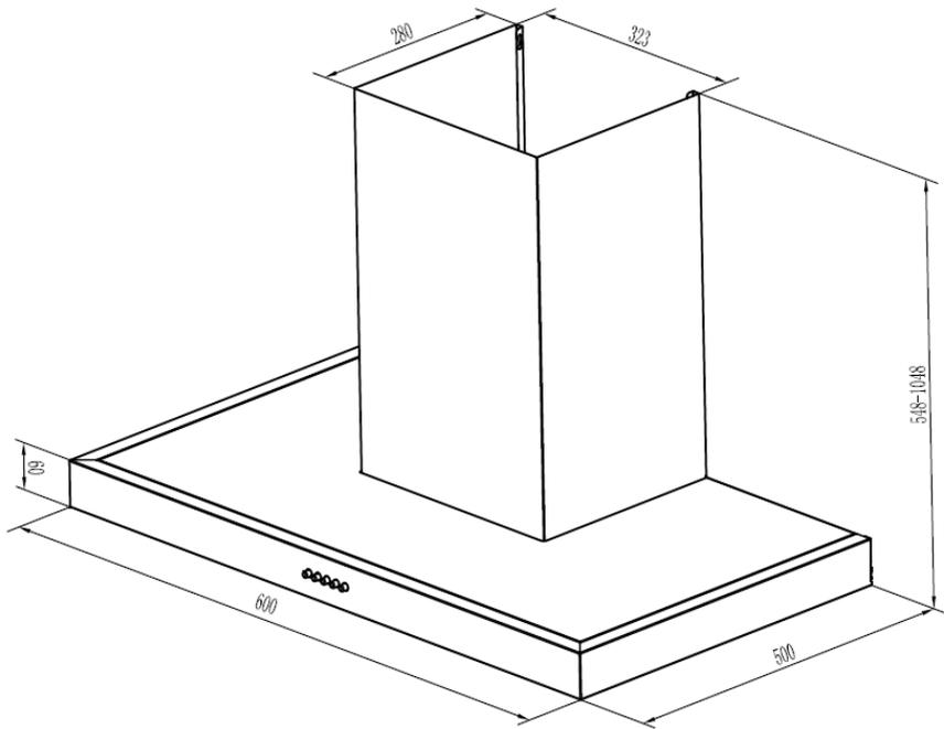
Abmessungen in mm.
