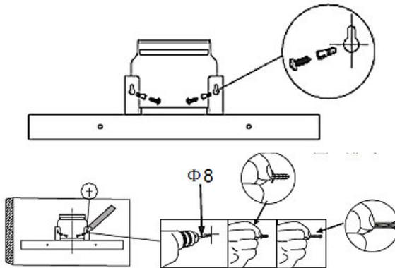
2. Suspend the appliance on the 2 installation openings and adjust it properly.
