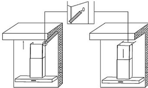
7. Install the fixing bracket on the corresponding position on the wall.
