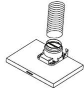
**Vertically:** Lay the exhaust hose to a roof cap\*.
