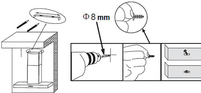
8. Fix the upper chimney using 4\*10 screws on the fixing bracket.
